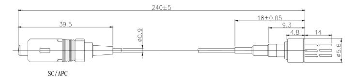
\*Note2: PIN orientation can be customized, Standard SC/APC connector and SMF pigtail, length is 17.5±0.5cm.
